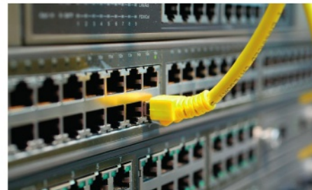
▲ Figure 5.10 A switch allows multiple devices to send data to each other
