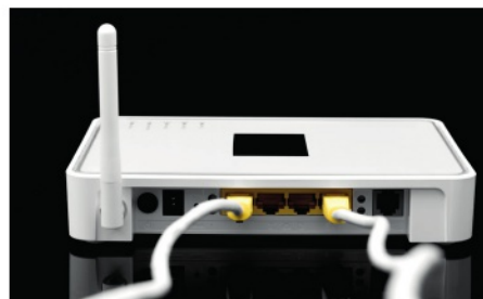
▲ Figure 5.12 This router has a four-port switch; the last (grey) port on the right is used to connect the router to a WAN (in this case, the internet)
