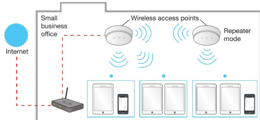
▲ Figure 5.9 Wireless access points can be used in a small business to provide Wi-Fi access to wireless devices in a network
