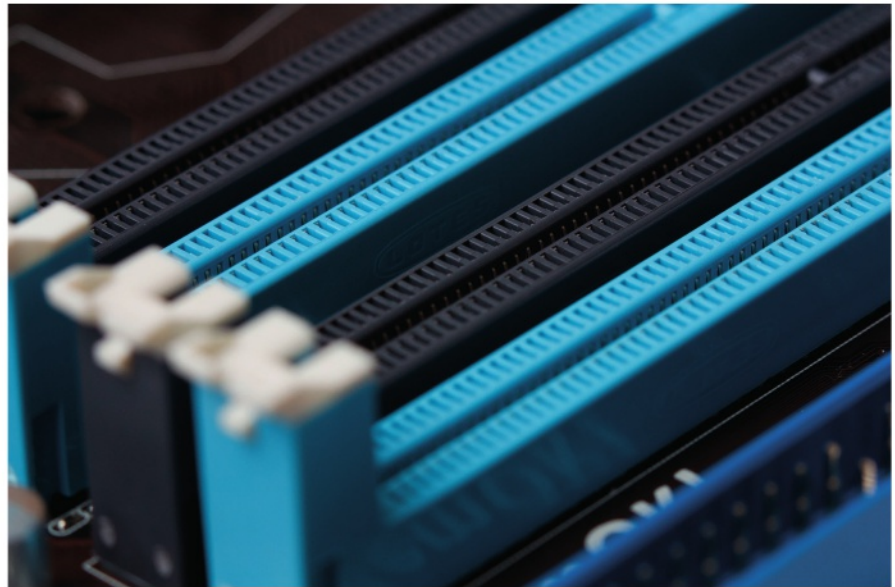
▲ Figure 3.2 A user can increase the amount of RAM using RAM slots on a motherboard
