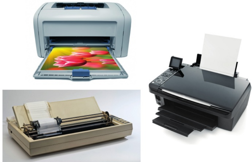
▲ Figure 1.62 Laser (top left), inkjet (right) and dot matrix (bottom left) printers
