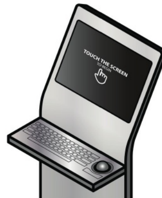
▲ Figure 1.39 Tracker balls are often used in installations like the kiosk shown here
