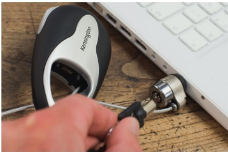
▲ Figure 1.33 A Kensington security lock in use
