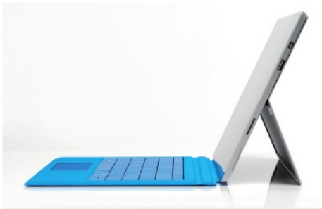
▲ Figure 1.23 Some tablet devices come with attachable keyboards, allowing them to operate as laptop computers
