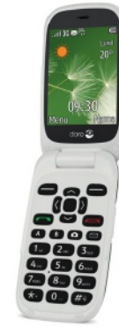
▲ Figure 1.9 Some mobile phones use tactile keypads, which are more responsive than other keypads, and give the user a choice of on-screen text size and colours
