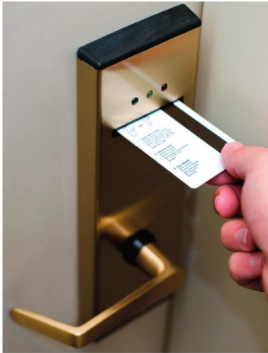
▲ Figure 1.56 Magnetic strip reader being used to unlock a door
