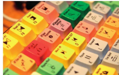
▲ Figure 1.36 This is an example of a keyboard used with specialist video software; the keys are mapped to specialist commands
